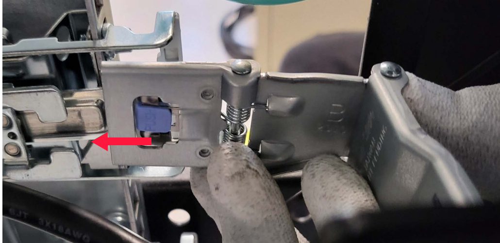
Figure 8.33 Aligning inner CMA arm connector and inner arm rail connector
