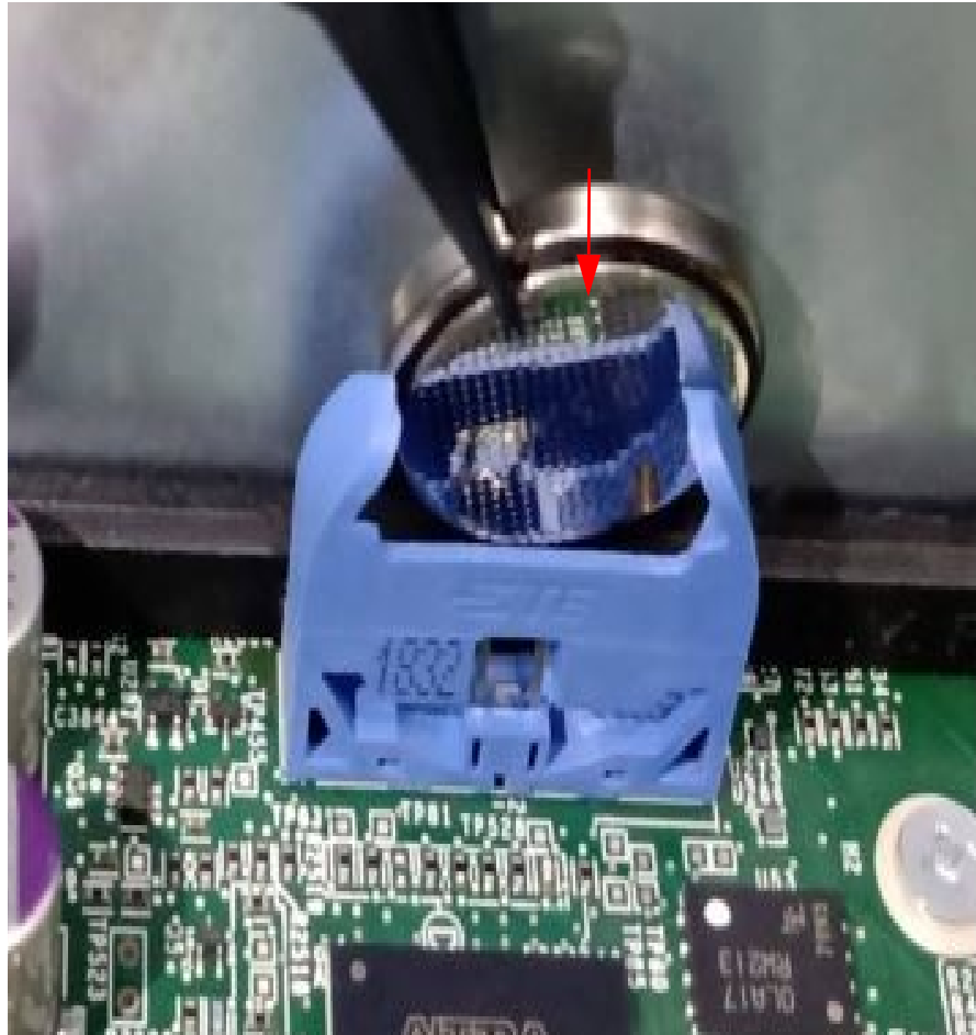
Figure 8.26 Positioning the replacement battery in the battery holder
