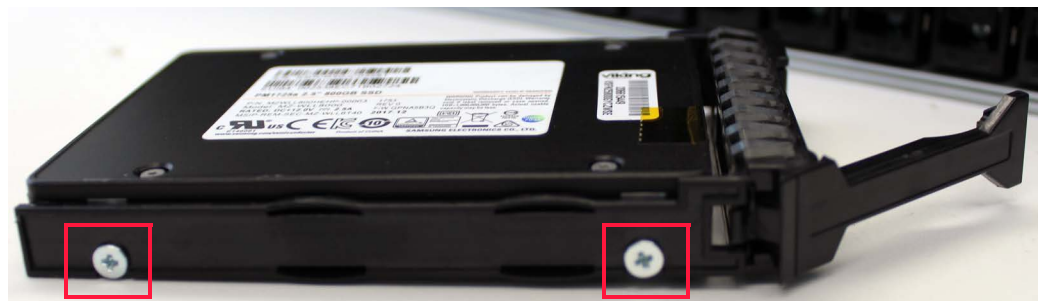
Figure 8.15 Drive carrier assembly screw location
