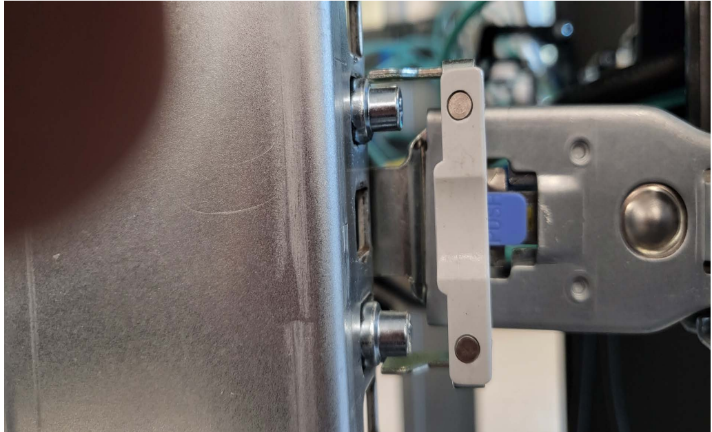
Figure 8.32 CMA body side correctly installed
