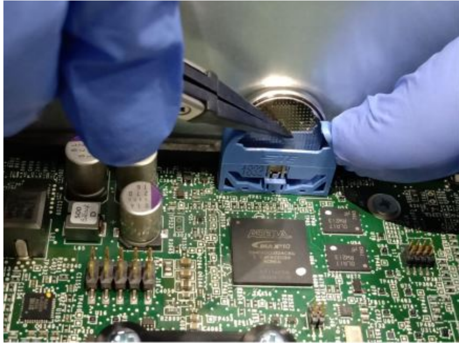
Figure 8.25 Pressing the battery out of the holder
